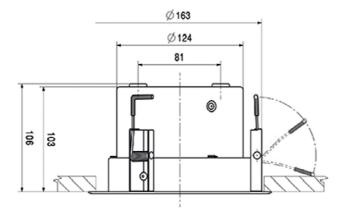
Measurements according to DIN IEC 268-5
